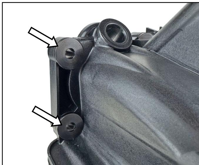
Secure intake manifold using supplied M6 x 25 Torx screws. **NOTE: Apply blue Loctite to threads. Torque bolts in sequence to 80 in•lb (9 N•m).**
