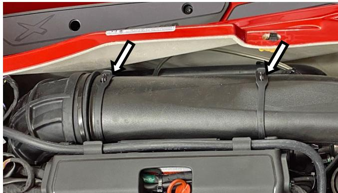
Remove plastic air intake tube. **TIP: Remove plastic clips on air intake tube cradle. They are easy to dislodge and they are not available separately!**
