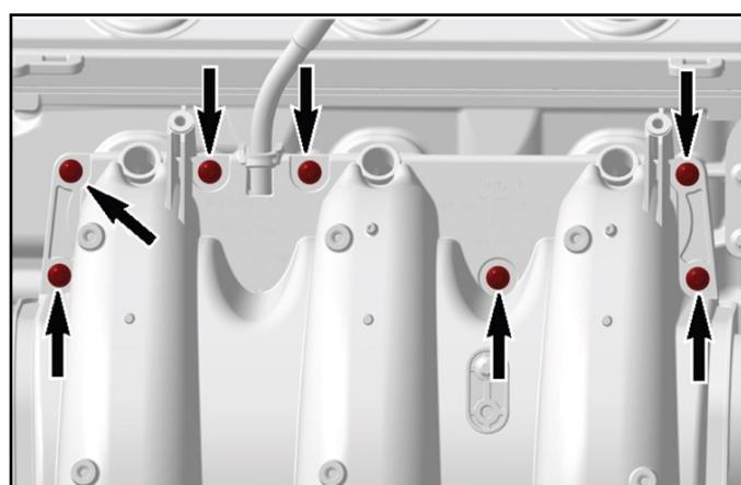
Carefully remove inserts (8) from intake manifold and discard.
